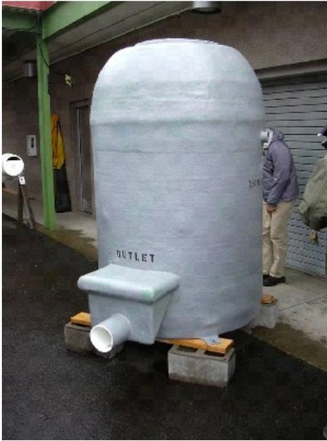
Manhole for accessing monitoring equipment
