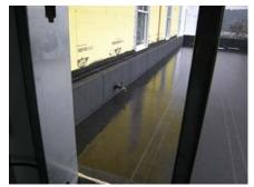
Testing waterproofing membrane May 2009
