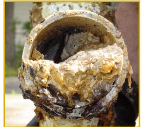
Grease clogged sewer pipe removed for cleaning.
