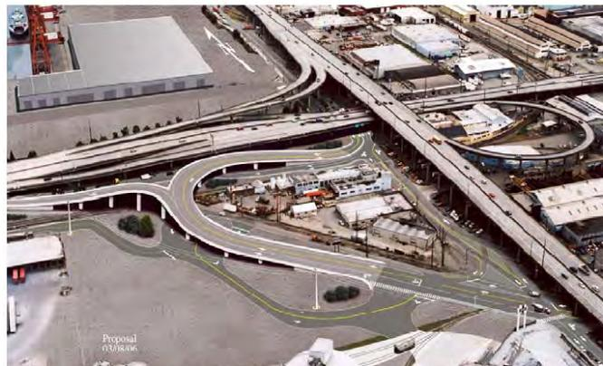
Figure 10: Grade Separated Intersection. Source: Port of Seattle.
