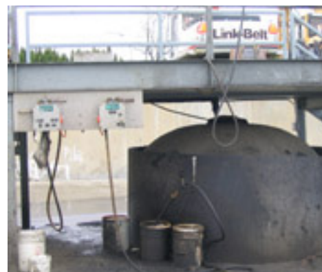
The PBOT Maintenance Operations program uses a soy-based product to prevent asphalt from sticking to tools and equipment.
