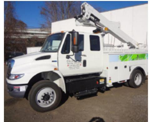
*This hybrid aerial bucket truck is one example of the hybrid utility vehicles used by CityFleet.*
