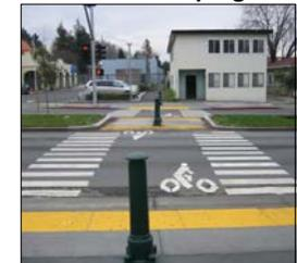
'Cross Bike' markings are a new type of marking used to highlight the presence of high volume bicycle crossings to passing motorists, similar to a crosswalk markings. Their use is currently under consideration by the City of Portland.
