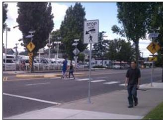
Rapid Flash Beacons are a new type of bicyclist or pedestrian activated beacon used to signal (flashing lights) to motorists the presence of a bicyclist or pedestrian waiting to cross. Research shows these devices to have motorist stopping compliance rates near that of a signal.
