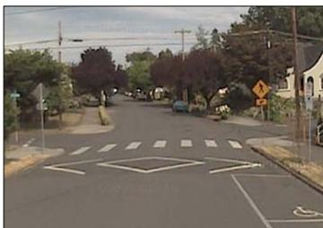
Speed bumps and pinch points and other traffic calming tools that slow traffic can have an added benefit of discouraging non-local traffic from using the street as a through route.
