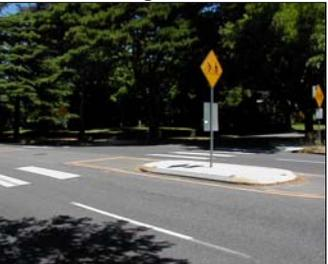
Median refuge islands reduce delay because the crossing distance for cyclists and pedestrians is shorter and the number of lanes to cross at one time is reduced, which increases the number of adequate gaps in traffic for safe crossings.
