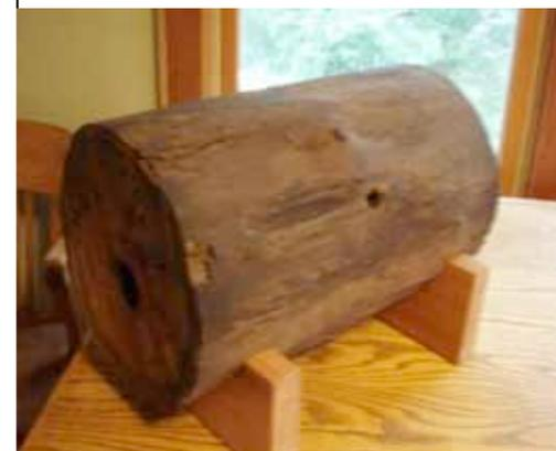
This example of Portland’s wood pipe is kept at Bear Creek House. The hole in the center is the main line. The hole in the side is an authorized service line, but this is also how buildings could secure themselves secret connections.
