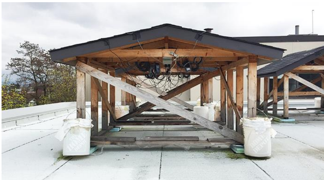
Figure 3: Roof hut decoupled from interior conditions by unrestricted ventilation to the underside of the roof sheathing. Monitoring equipment was installed to measure performance characteristics including sheathing moisture content at various depths, roof surface temperature, sheathing temperature, and ambient temperature and relative humidity.
