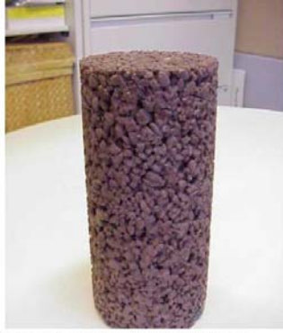
Core-Sample of Pervious Concrete, Dyed Brown
