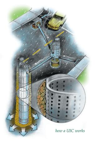
ment facilities often overflow to UICs. That keeps stormwater runoff in the watershed, out of sewers, and reduces stormwater discharges to rivers and streams.
