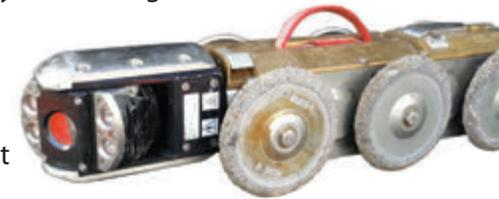
**Remote-controlled cameras are used to inspect sewer pipes.**
