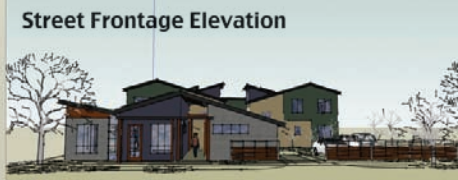
Street Frontage Elevation Street frontage features a sliding gate and screen fence with low wood panels (to 3' ht.) with taller steel frame, presenting a porous, pedestrian-scale screen for neighbors. Cars stopping to open gate before entering makes for a safer pedestrian zone.
