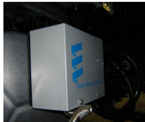
A diesel coolant heater warms a vehicle's engine prior to starting, reducing idling time.
