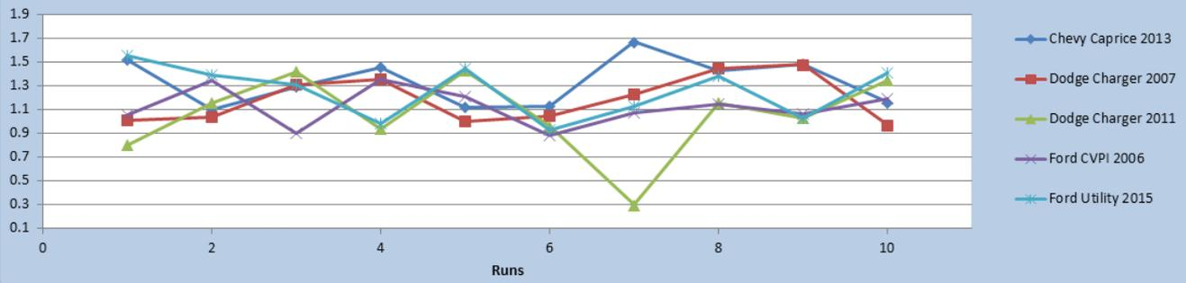
Figure 3. Impact of ESC on Time of Rotation: J-Turn
