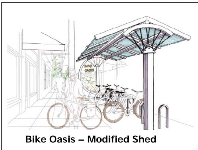
Subcommittee members gave additional input to Browning-Shono on the overall design of bike oasis, focusing on the roof, columns and materials. Browning-Shono then developed a Modified Shed Scheme for the subcommittee's review. The design uses mini-staple type bike racks and the column with the bicycle spokes at the top resembles a papyrus column. The roof will be transparent to let
