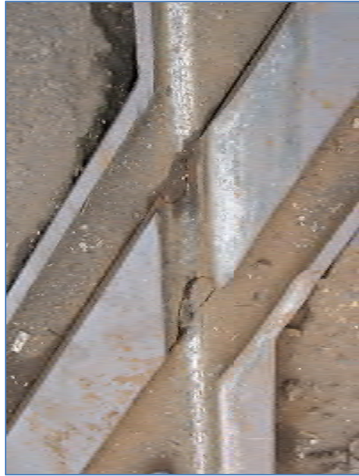
Figure 5: Left: Railcar wheel flange incising into crossing frog up to 3/4" deep. Right: Chipping and cracking in crane rail at crossing frog.
