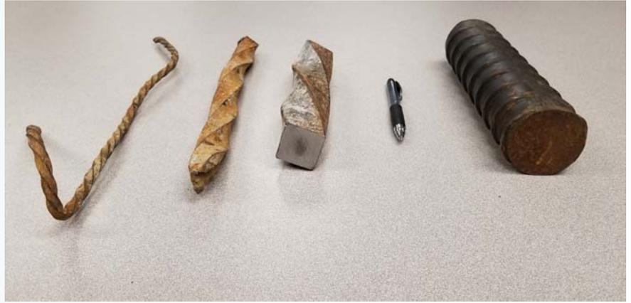
Rebar, a standard element used to strengthen concrete in structures, has evolved over the years, as well as how it's used. The three examples on the left (above photo) have been harvested while demolishing the historic structure. Rebar was used very sparingly during that construction, often spaced feet apart. To the right is an example of the rebar in use for this project, spaced only inches apart. We receive and store a lot of rebar and use it everywhere.
